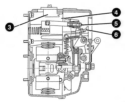
\* Lug cam with torque control
